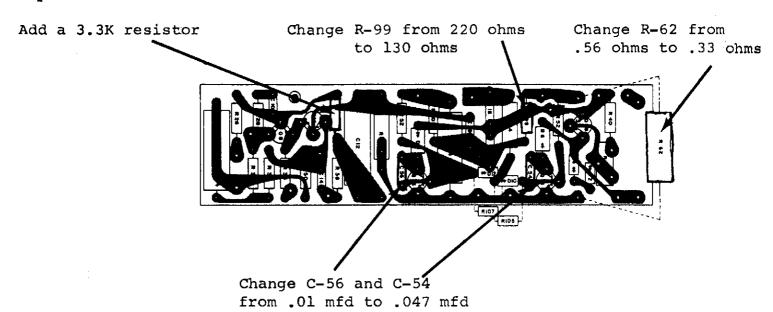
The right channel power output printed circuit board is shown. Do likewise on the left channel board.
